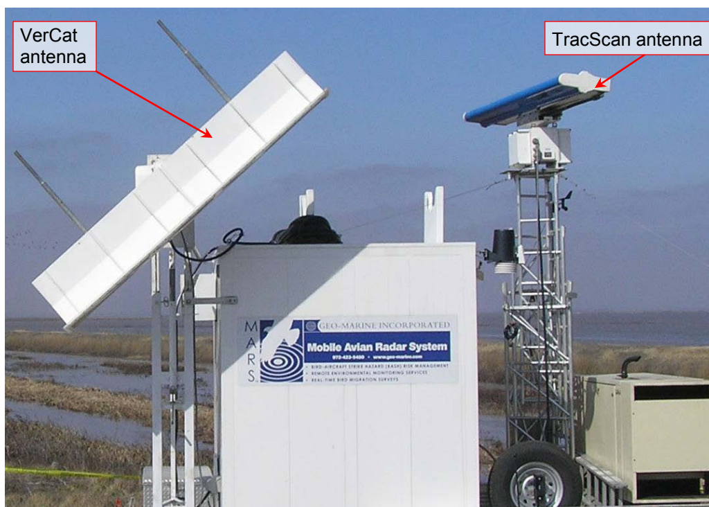
Figure 5-1. GMI MARS ® showing both VerCat and TracScan antennae and transmitter/ receiver units.
